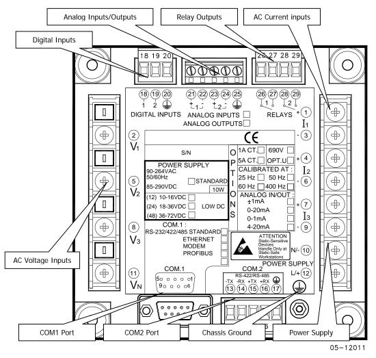
Figure 6: Connections and Terminals
