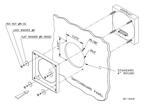
Figure 2 (ANSI 4" round cutout): Mounting the display unit
