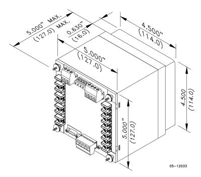
Figure 1: Instrument Dimensions
