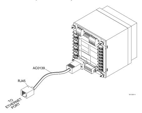
Figure 11 COM1: Ethernet Connection
