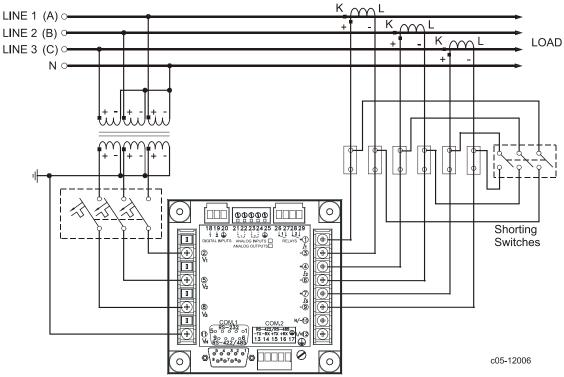
Figure 7: Typical Installation 2
