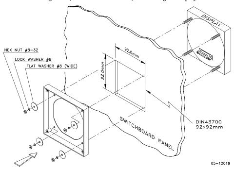
Figure 3 (DIN 92x92mm square cutout): Mounting the display unit
