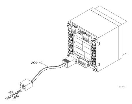
Figure 10 COM1: Telephone Line Connection
