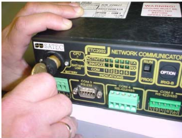
Figure 7-4 Insertion of New Battery
