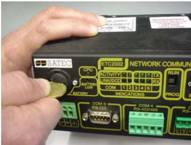
Figure 7-2 Battery Housing Cover Removal
