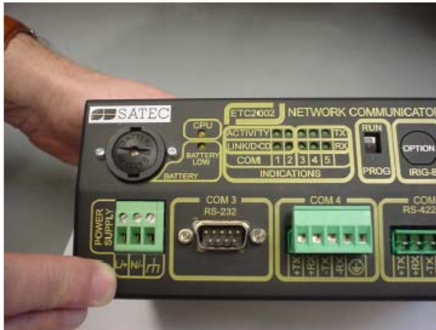
Figure 7-1 Battery Housing Location of the Panel
